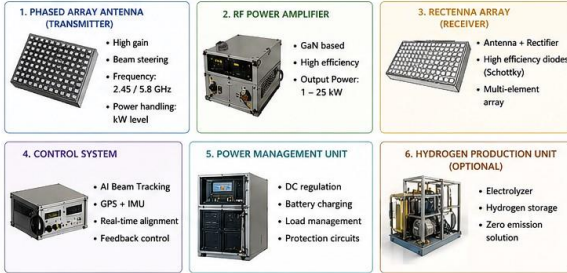
Figure 3: Major Equipment of MWPT System
