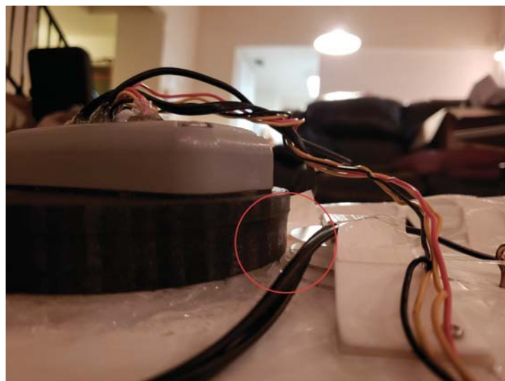
Figure A.4: Snapshot showing clearance of rear sail spool.
